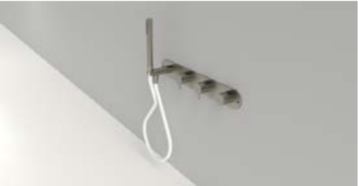
Gruppo doccia incasso termostatico, collettore due vie, rubinetto di chiusura, flessibile e doccia (raccordo 3/4") Horizontal built-in shower group made of thermostatic mixer, two ways manifold, stop valve, hand shower and flexible hose (3/4" connection)
