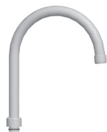
ZCANA020 Canna tubo ombrello, Ø 20 mm interasse 185 mm, con aeratore, per art. 180 Complete tube spout Ø 20 mm with aerator for art. 180, distance between centres 185 mm
